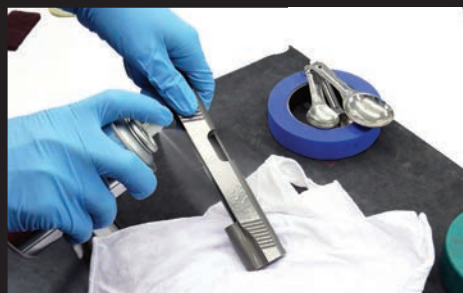
1st. Degrease with TruStrip™
