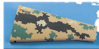
Step 8 Remove female templates and apply DuraCoat® Clear.
