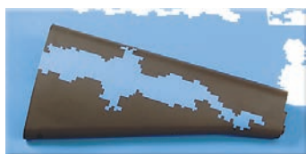
Step 1 Randomly select one or more Peel 'N Spray™ templates and place on the base coated item.
