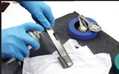
1st. Degrease with TruStrip™
